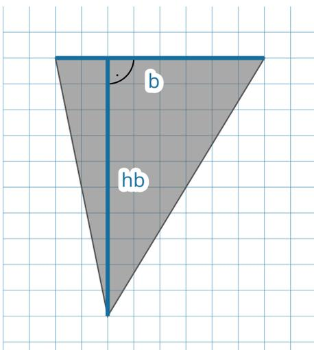
$$\begin{aligned} A_{\Delta} &= \frac{b \cdot h_b}{2} \\ &= \frac{4\text{cm} \cdot 5\text{cm}}{2} \\ &= \frac{20\text{cm}^2}{2} \\ &= \underline{\underline{10\text{cm}^2}} \end{aligned}$$
