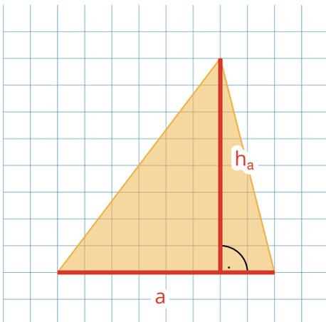
$$\begin{aligned} A_{\Delta} &= \frac{a \cdot h_a}{2} \\ &= \frac{4\text{cm} \cdot 4\text{cm}}{2} \\ &= \frac{16\text{cm}^2}{2} \\ &= \underline{\underline{8\text{cm}^2}} \end{aligned}$$
